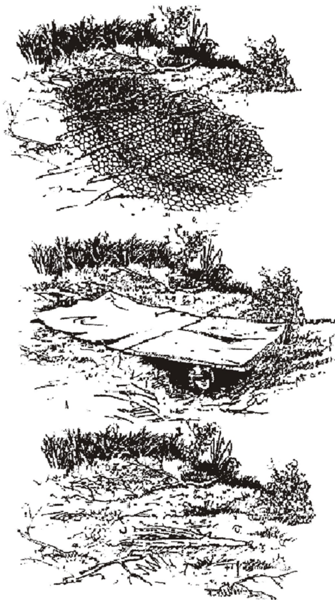
Figure 11-2: Construction of an OP—Option 1
